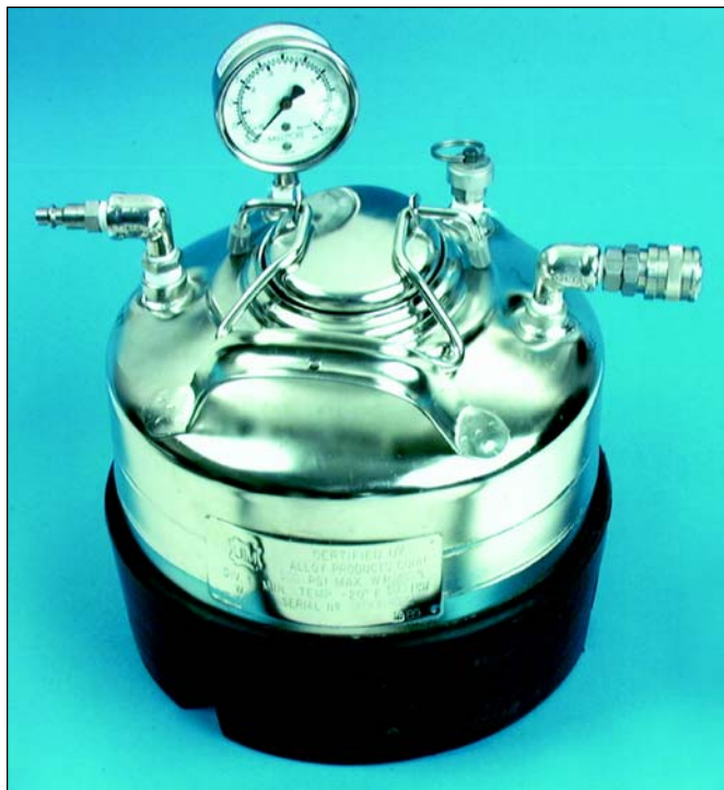
Figure 3. Pressure can with dip tube removed and 'quick disconnect' connections added.
