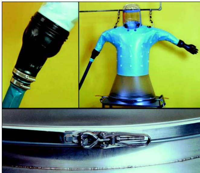
Figure 4. Inflated half-suit. Note the yellow test cloth in the helmet, and close-up of modified glove/exhaust line and close-up of 'high' clamping of the suit to the inflation plate.
