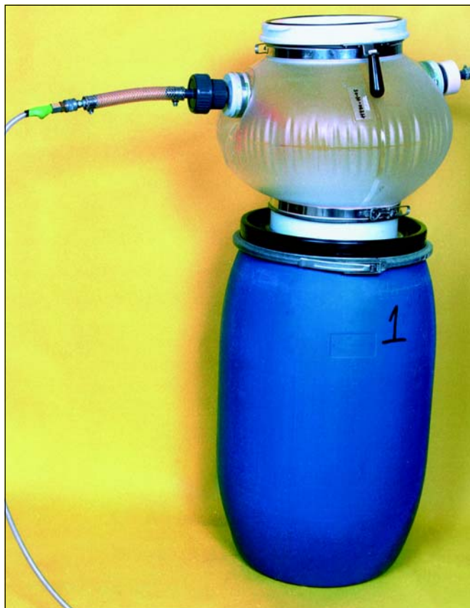
Figure 5. Inflated waste container. Air inlet connector is on the left and the sterilization exhaust is on the right.
