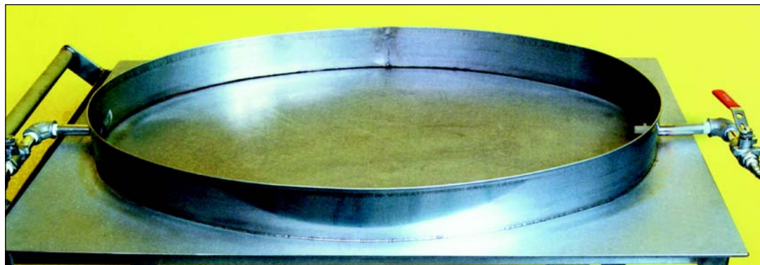
Figure 1. Inflation plate for half-suits. Note inlet valve on right with 'quick disconnect' connector.
