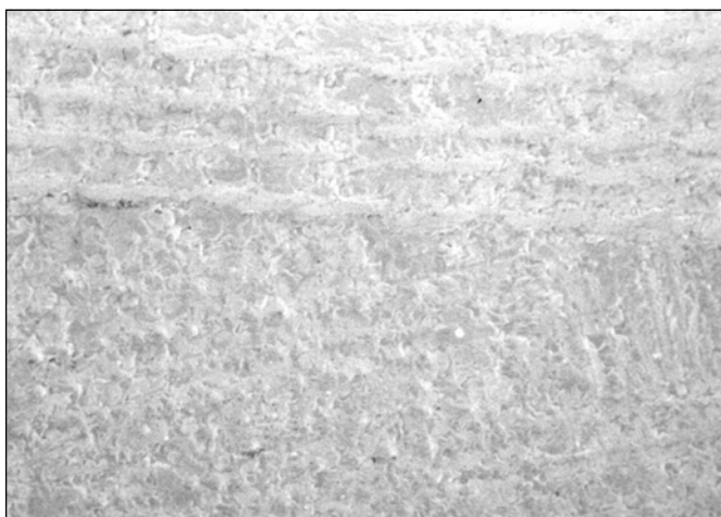
Figure 4. Low magnification view (470X) of light area on inside of tube weld.
