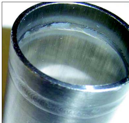
Figure 1. Visual discoloration on welds.
