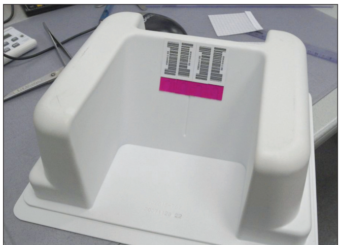
Figure 5. Specially shaped reference tub with dose sensitive strips. 2
