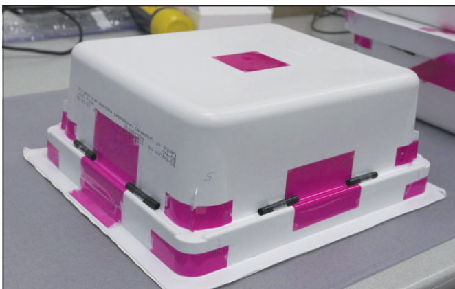
Figure 4. Low dose point determination using dose mapping with radio-chromatic film (tub is shown upside down to allow view of tub underside). Pink color of film indicates the tub was exposed to radiation.
