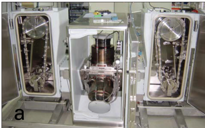
Figures 2a and 2b. E-beam tunnel view (shielding panels removed, transport labyrinth shown left and right, emitter arrangement shown in center).
