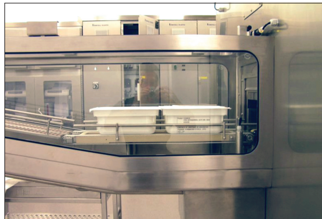
Figure 9. E-beam tunnel tub infeed.
