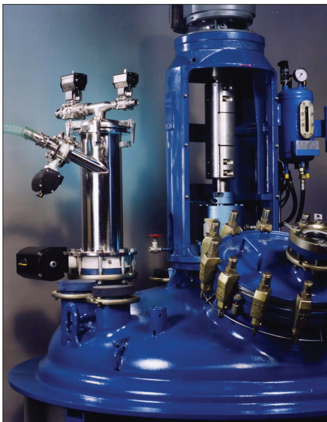
Figure 9. Powder Transfer System.
