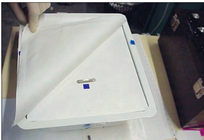
Figure 7. Additional Tyvek sheet under lid (liner).
