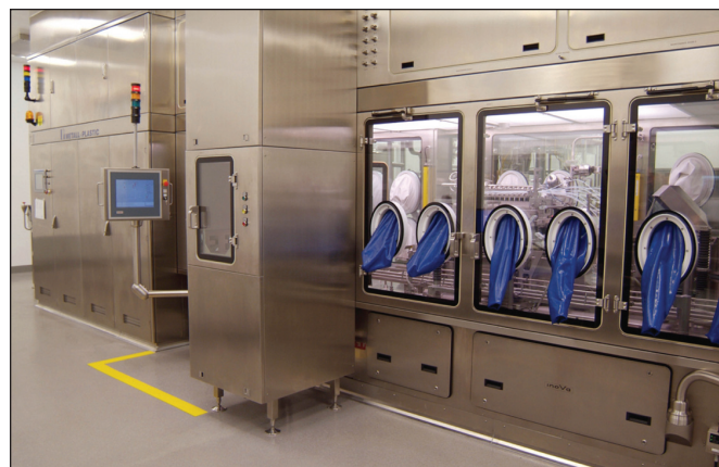
Figure 10. Isolated syringe filling line. Output: 350 syringes per minute.
