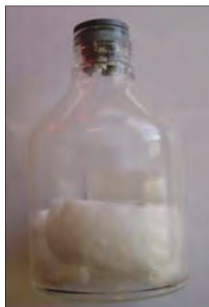
Figure 2. One liter glass bottle after freeze-drying with a fill weight of 400ml.
