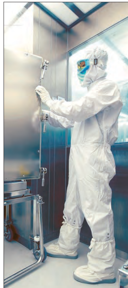
Cleanroom operator opening the cabinet containing sterilized frames for the freeze dryer.
