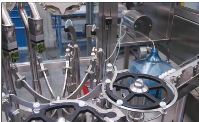
Aseptic Technologies: Filling and laser re-sealing in capping area of workshop.
