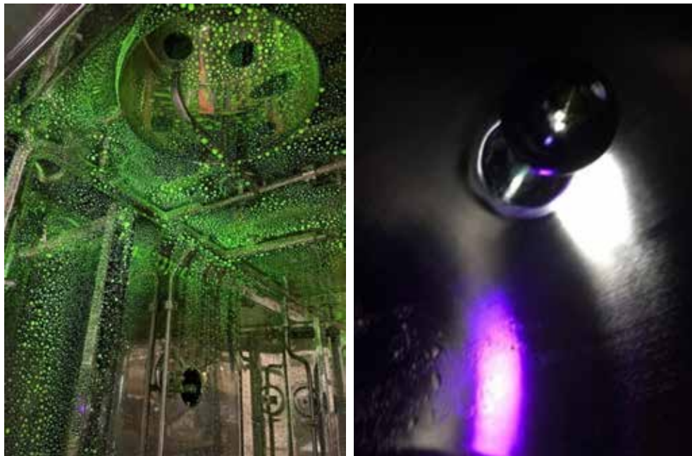
Figure 3: Example of spray coverage image and clean in place (CIP) execution image used as supporting evidence.
