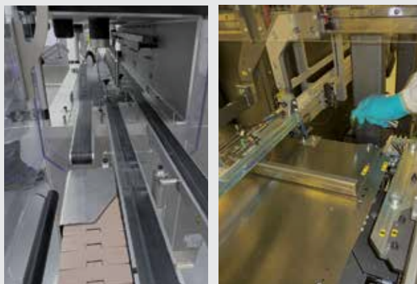
Figure 2: Potential areas of entrapment within packaging equipment
