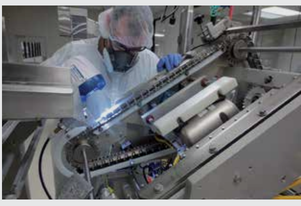
Figure 5: QA inspection of disassembled slat-style bottle filler
