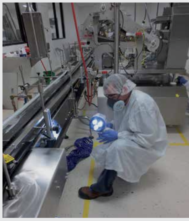
Figure 4: Inspection method: Use of additional lighting
