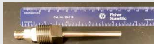
Figure 1: Fitting used for connection to tubing. Fitting was machined to an external diameter equal to the ¼-inch internal tubing diameter.
