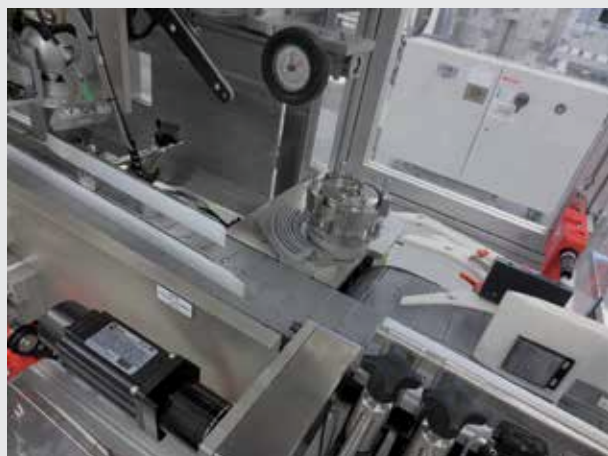
Figure 3: Pinch points on a typical packaging machine
