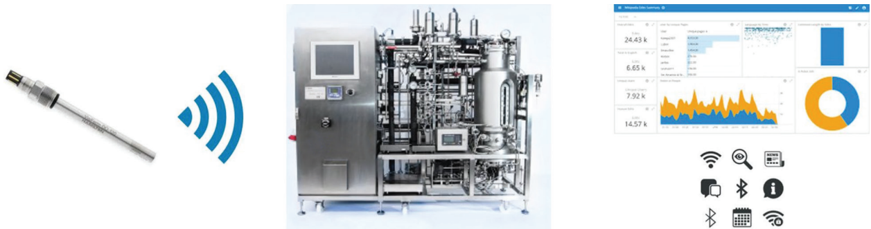
Figure 3.1: Schematic Representation of the PoC Smart Sensor (left), Bioreactor (center), and Cloud Cockpit (right)
