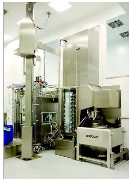
Compression operation (incl. PAT application).
