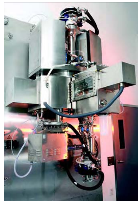
Isolated single pot process with dryer and isolated automated sampler.
