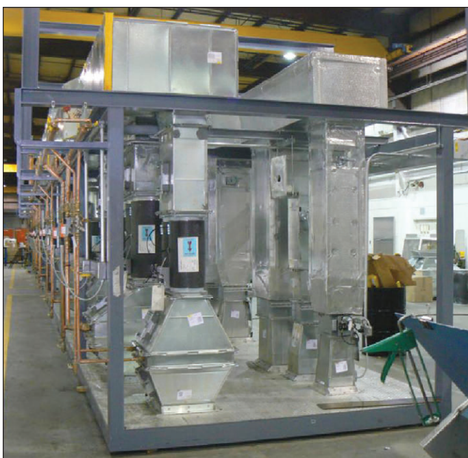
Ductwork riser skid.
